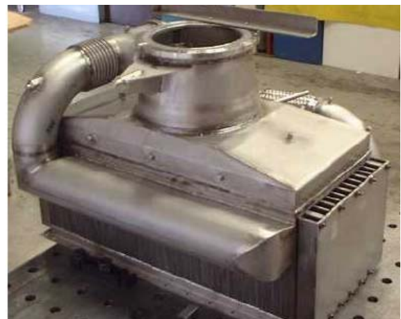
Figure 2.5: A Counter Flow Recuperator (from ref. [10]).
