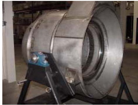
Figure 2.4: Annular Recuperator for a 200 kW MGT (from ref. [15]).
