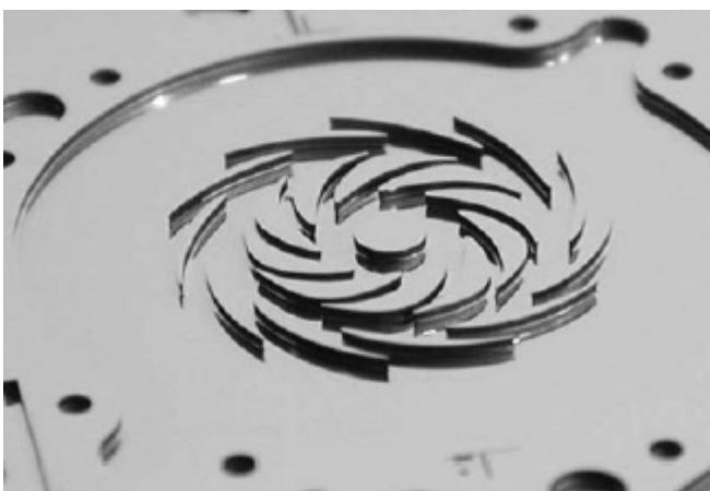
Figure 2.20: Centrifugal Flow Compressor and Radial Inflow Turbine on Micro-Scale (from ref. [39]).
